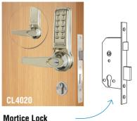
Furo profile mortice sash lock with deadbolt and latchbolt. With the deadbolt thrown it denies access to code users. Supplied with Euro profile cylinders and three keys.
